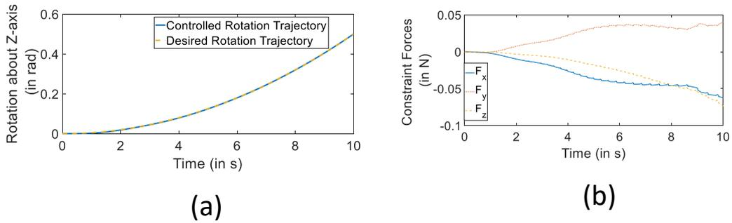
Figure 1: (a) The desired rotation of the object and the controlled trajectory in the z-axis (b) Corresponding reaction forces
