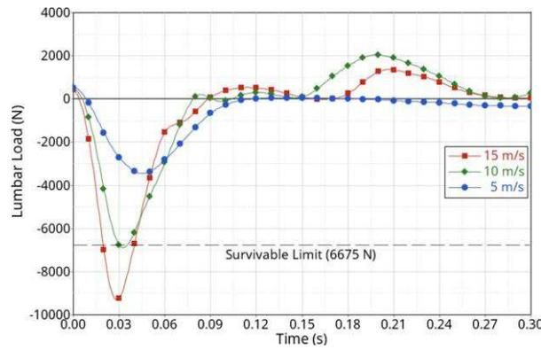
Figure 2: ATD lumbar load for different drop velocities in one structural configuration
