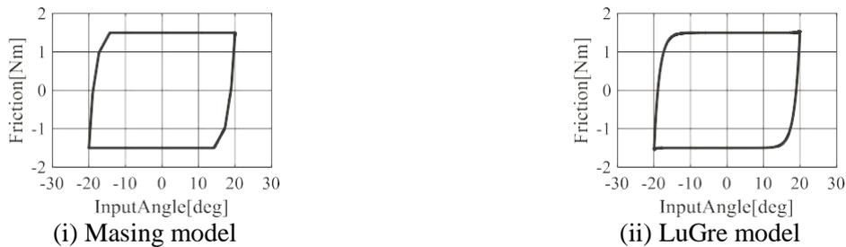
Figure 4: Characteristics of friction models
