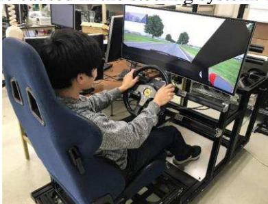
Figure 1: Steering torque simulator
