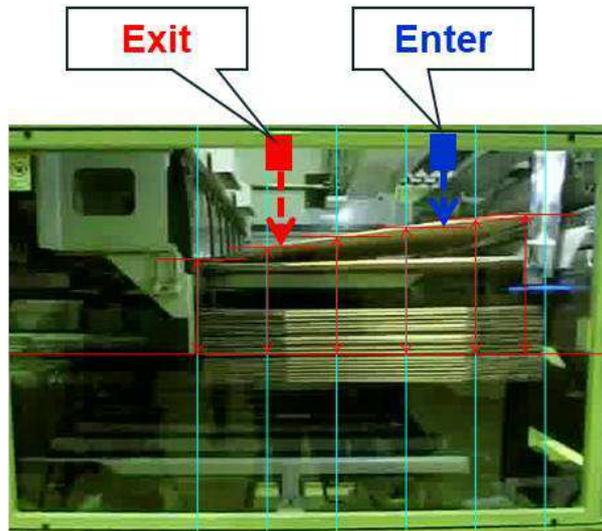
Figure 3: Deformation measurement through laser-sensor and video capture
