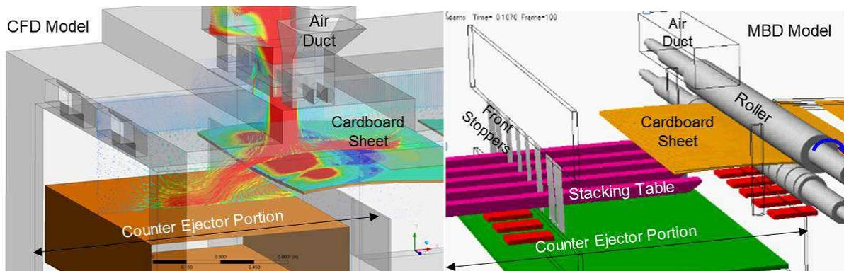
Figure 2: Representative CFD and MBD model of cardboard passing through counter ejector
