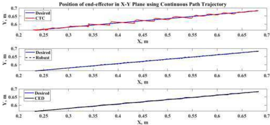
Fig. 1: Comparison of positions of end-effector of Two-Link Flexible manipulator [7] in X-Y Plane obeying Continuous path trajectory: obtained by using different controllers
