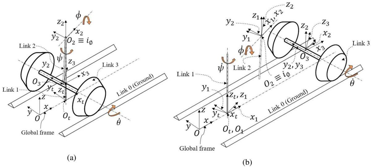
Figure 1: (a) Serial chain wheelset model, (b) Exploded view of serial chain model
