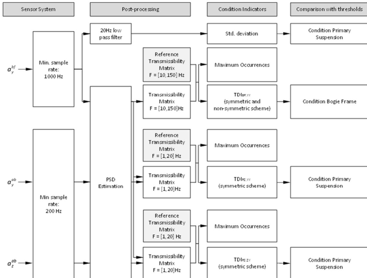
Figure 2: Data flow for the condition monitoring methods
