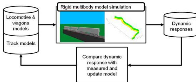
Figure 1: Comparative study of the model behavior against experimentally acquired dynamic responses
