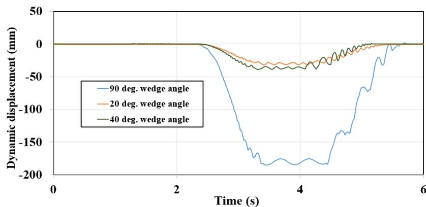
Figure 2: Comparative dynamic sag of the frontal link in linear chain
