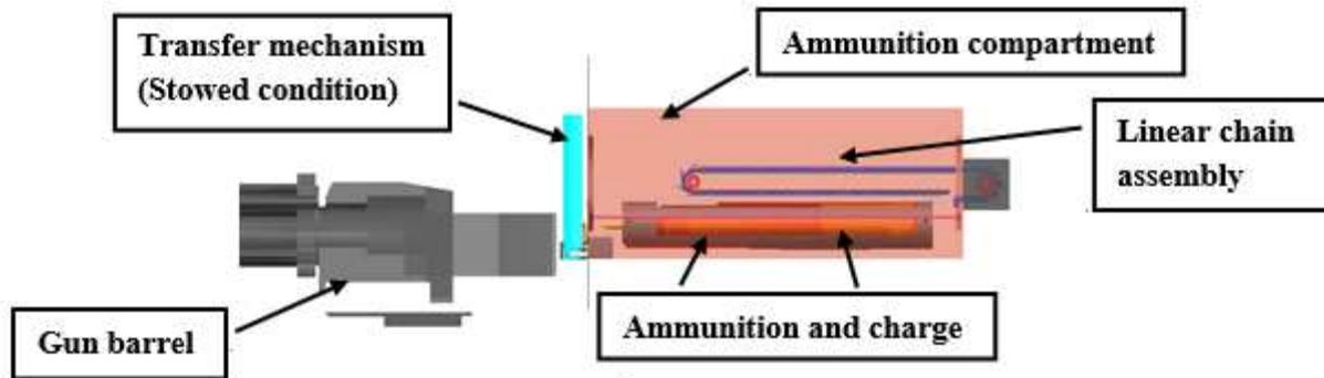
Figure 1: Schematic representation of the Autoloader assembly
