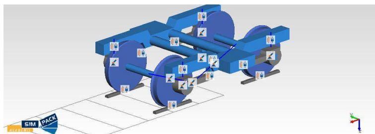
Figure 1: Simulation model of a bolsterless bogie (electric motored)
