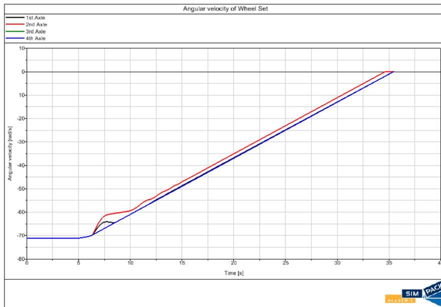
Figure 3: Angular velocity of wheel sets
