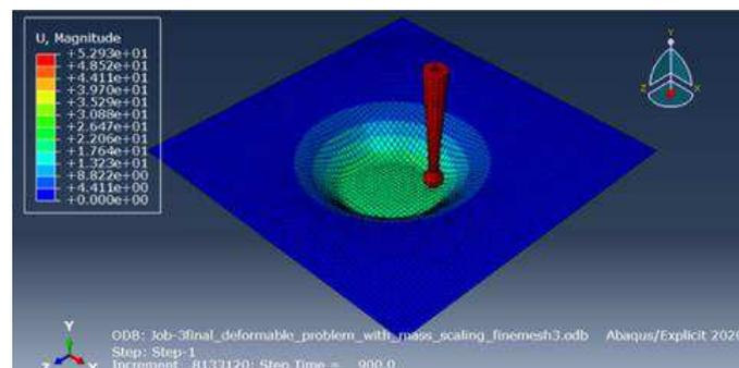
Figure 2: Deformation profile of truncated cone in SPIF process with a deformable tool.
