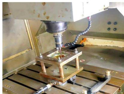
Figure 1: SPIF process on Jyoti Huron KMill CNC machining centre
