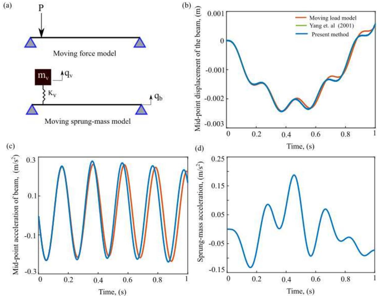
Figure 1: (a) Idealisation of moving load and sprung-mass model over simply-supported beam; (b) Mid-point displacement of the beam; (c) Mid-point acceleration of the beam; and (d) Acceleration response of the sprung mass system.
