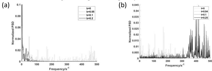
Figure 2. Spectrum-power density distributions of sun gear, (a) different clearances; (b) different tolerances.
