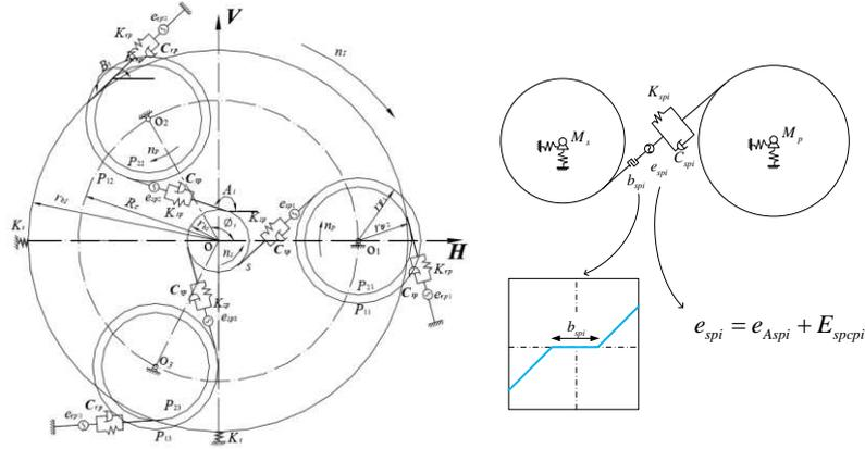
Figure 1. The lump-mass parameter model for the planetary spur gear system.
