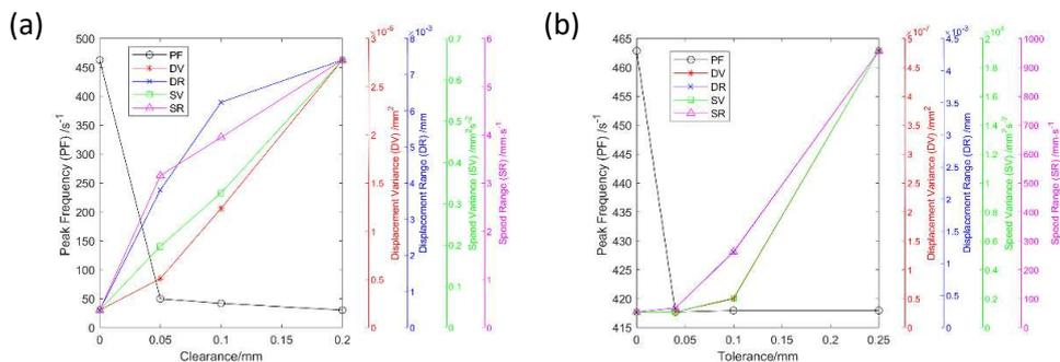
Figure 3. Vibration response parameters of sun gear rotation response, (a) different clearances; (b) different tolerances.
