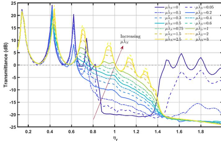
Figure 3: Transmittance with respect to frequency ratio ( $\eta_r$ ) plot for the 7<sup>th</sup> unit in the metamaterial chain for varying non dimensional maximum frictional force ( $\mu \tilde{\lambda}_N$ )
