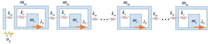
Figure 2: A metamaterial chain comprising of finite number of mass-in-mass frictional unit cells
