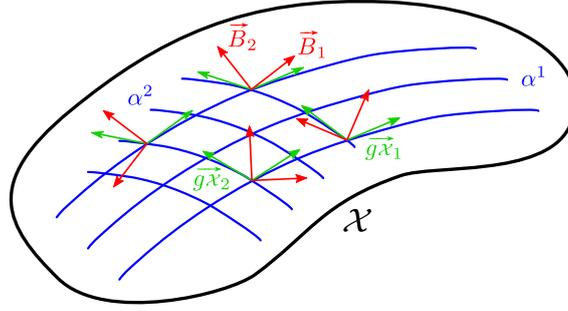
Figure 1: Local orthonormal bases  $B(\bar{\alpha}, t)$  made of basis vectors  $\vec{B}_i(\bar{\alpha}, t)$  introduced on the current configuration  $\mathcal{X}$  of a flexible body. The convected coordinate lines are denoted by  $\alpha$  and the base vectors tangent to these coordinate lines are denoted  $\vec{g}_{\mathcal{X}_I}(\bar{\alpha})$ .
