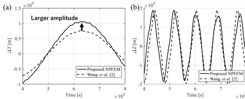
Fig. 2 Comparison of displacements of tether free end at climber ascent (a)  $Y$ -direction, (b)  $Z$ -direction
