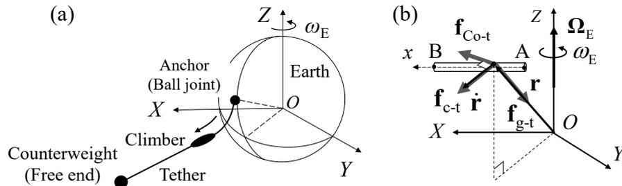
Fig. 1 (a) Components of non-equatorial space elevator and coordinate system (b) Gravitational force  $\mathbf{f}_{g-t}$ , centrifugal force vector  $\mathbf{f}_{c-t}$ , and Coriolis force vector  $\mathbf{f}_{Co-t}$  acting on arbitrary point in tether element
