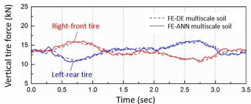
Figure 2: Vertical tire forces of lane change maneuver simulation using the FE-ANN multiscale terrain model. The results are in good agreement with those of the FE-DE multiscale model.
