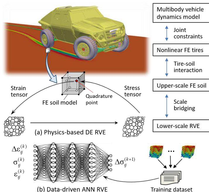
Figure 1: Multiscale off-road mobility simulation framework
