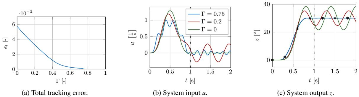
Figure 2: Numerical results for inversion of the flexible manipulator with one link with redefined system output  $\tilde{z}$ .
