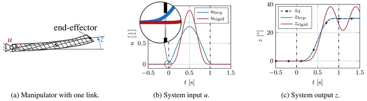
Figure 1: Model and numerical results for system inversion for a flexible manipulator with one link.
