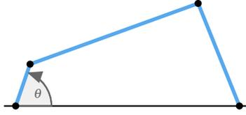
Fig. 1 Four-bar linkage.
