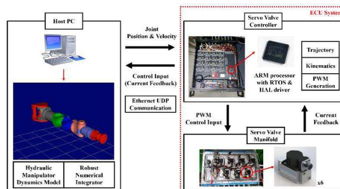
Figure 1: Configuration of hydraulic manipulator HILS simulator.
