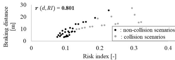
Figure 3: Correlation between risk index of test scenarios and braking distances.
