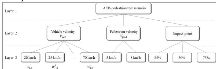
Figure 2: Hierarchy model of AEBS-pedestrian test scenario.
