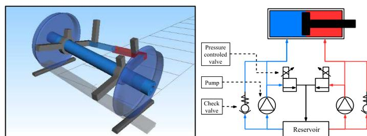
Figure 1: Running gear SIMPACK implementation (Left) and actuator schematic (Right)
