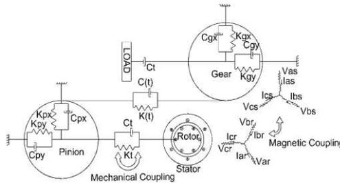
Fig. 2. Coupled electromechanical modelling of gearbox
