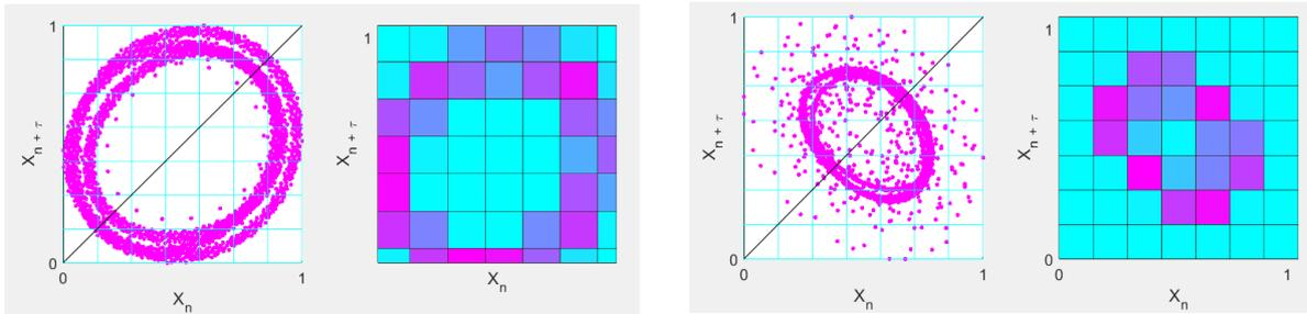
Fig. 5 Poincaré plot and bivariate histogram of the grid point distribution based on the healthy and tooth crack 2.64 mm at VMF1-TSA of 10000 datapoints
