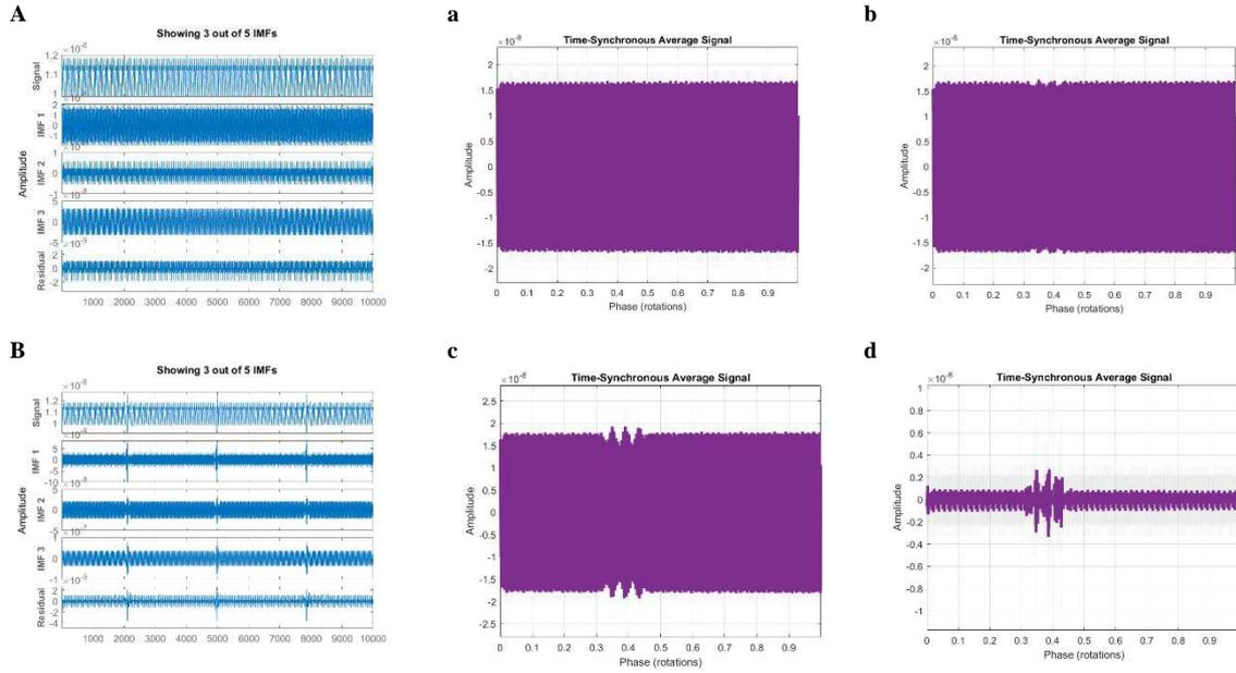
Fig. 4. (A) VMD-IMFs of healthy tooth (B) VMD-IMFs of tooth crack at 2.6 mm (a) VMF-TSA of healthy tooth (b) VMF-TSA of tooth crack 0.08 mm (c) VMF-TSA of tooth crack 1.76 mm and (d) VMF-TSA of tooth crack 2.64 mm
