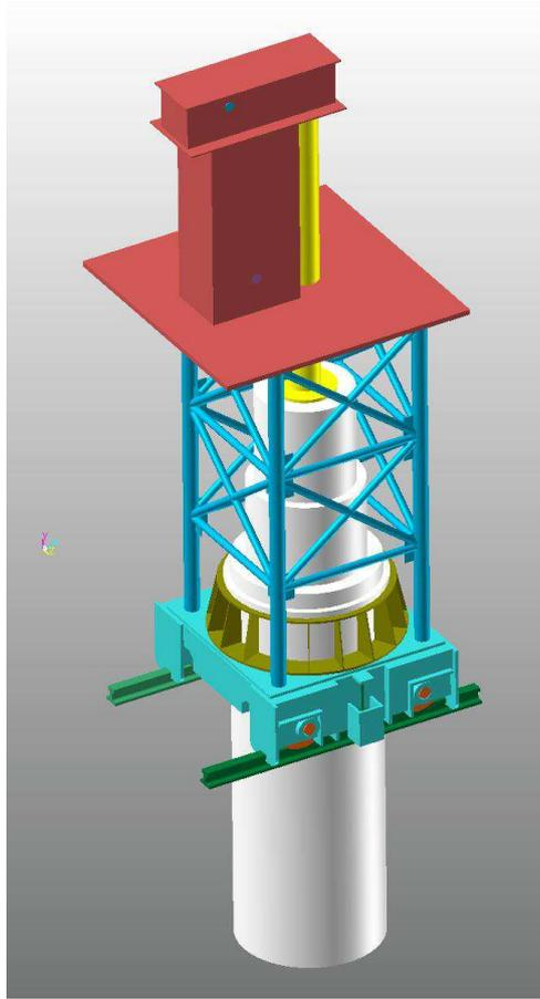
Figure 1: Docked Sub Assembly Transfer Flask
