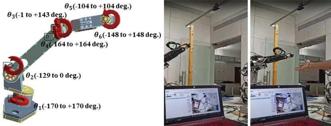
**Fig. 2. a.** Joint angle limits of the open source robot arm, **2. b.** Human robot collaboration
