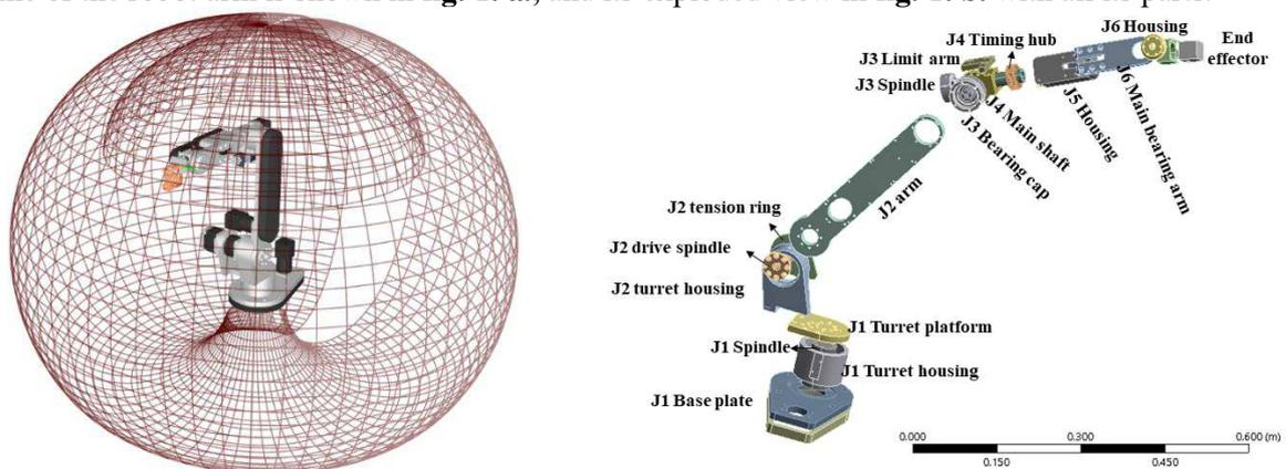
**Fig. 1. a.** AR3 robot workspace visualization, **1. b.** Exploded view of the assembled robot arm
