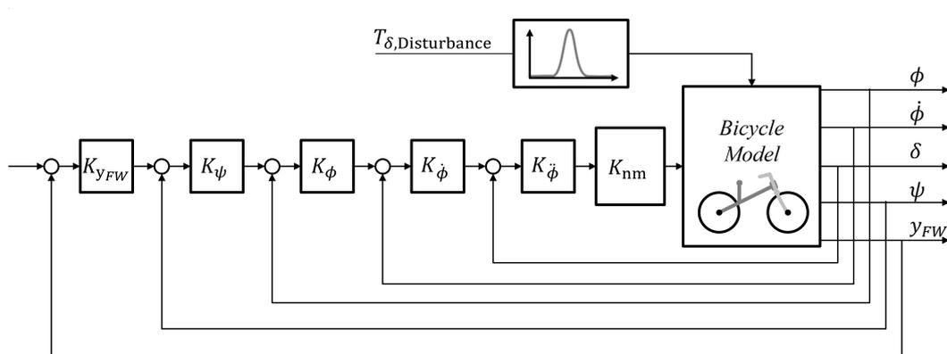
Figure 1: Closed-loop multibody simulation setup [5, 6].
