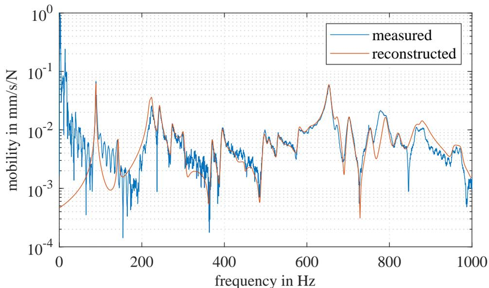
Figure 2: Comparison of measured mobility and mobility reconstructed from an experimental modal analysis for a point on the soundboard below the bridge.
