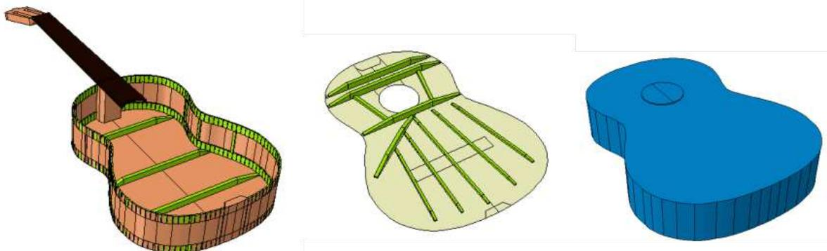
Figure 1: Finite element model of the guitar. The colors visualize the different materials of the guitar and the most right picture displays the simplified air volume inside the guitar.
