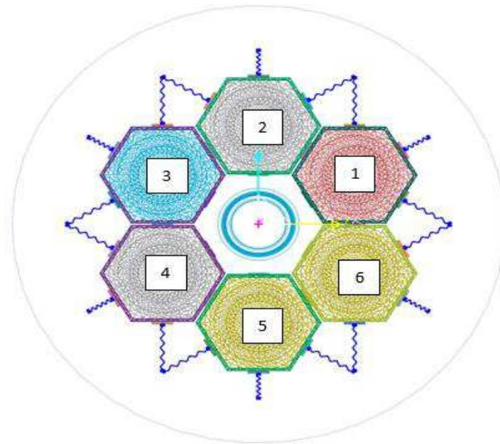
Figure 1: Schematic diagram of adjacent SAs with spacer pads and spring elements
