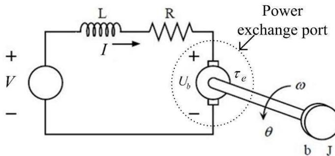
Figure 1: Equivalent circuit of a DC motor
