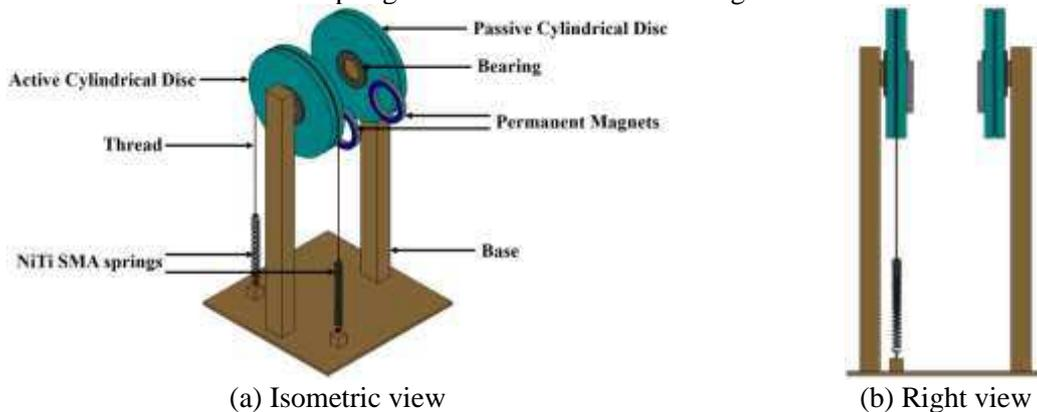
Figure 1. Proposed permanent magnet based SMA operated actuator.
