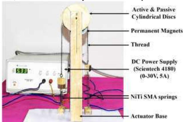
Figure 2. Experimental Setup of the proposed novel actuator.
