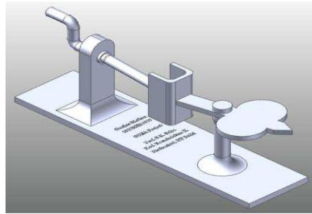
Figure 2: CAD model of the synthesized mechanism
