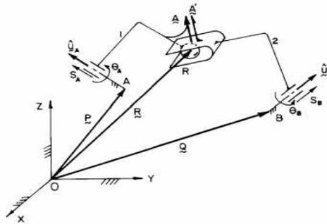
Figure 1: Schematic of R-Sp-R Mechanism [2]
