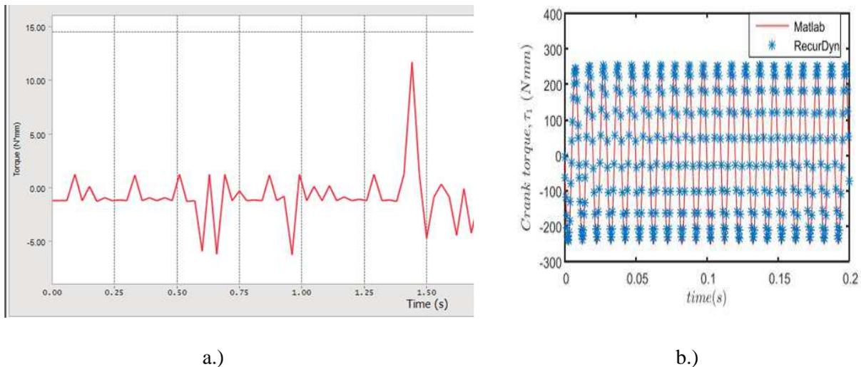
Figure 3: Torque(N\*mm) vs Time(s) curve for: a.) Synthesized mechanism b.) Existing mechanism [1]
