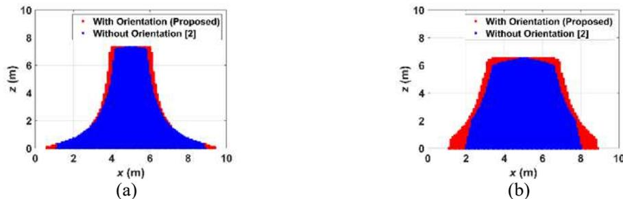
Figure 3: Effect of orientation on the printable workspace for (a) case 1 and (b) case 2
