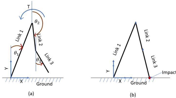
Figure 1: Kinematic structure of the biped system: (a) during swing phase (b) during ground impact.
