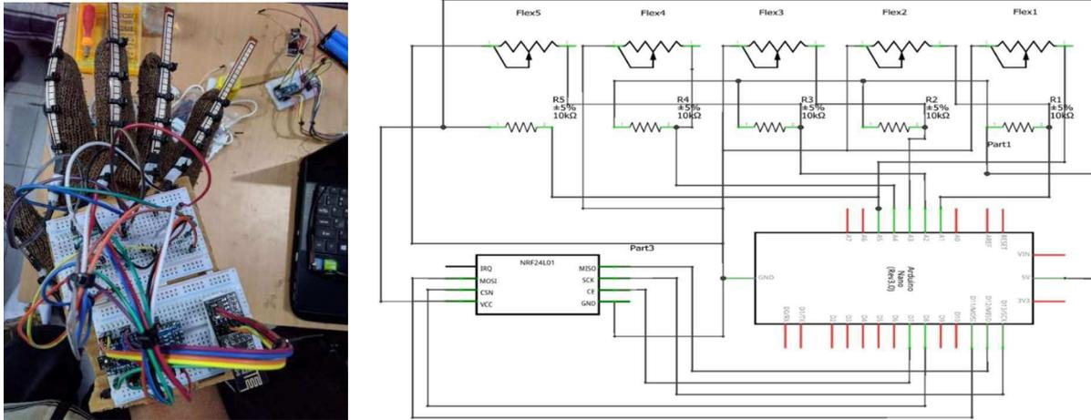
Figure 2: Controller Glove, actual image (left) and schema diagram (right).
