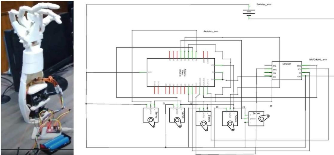
Figure 3: Robotic Hand, actual image (left) and schema diagram (right).
