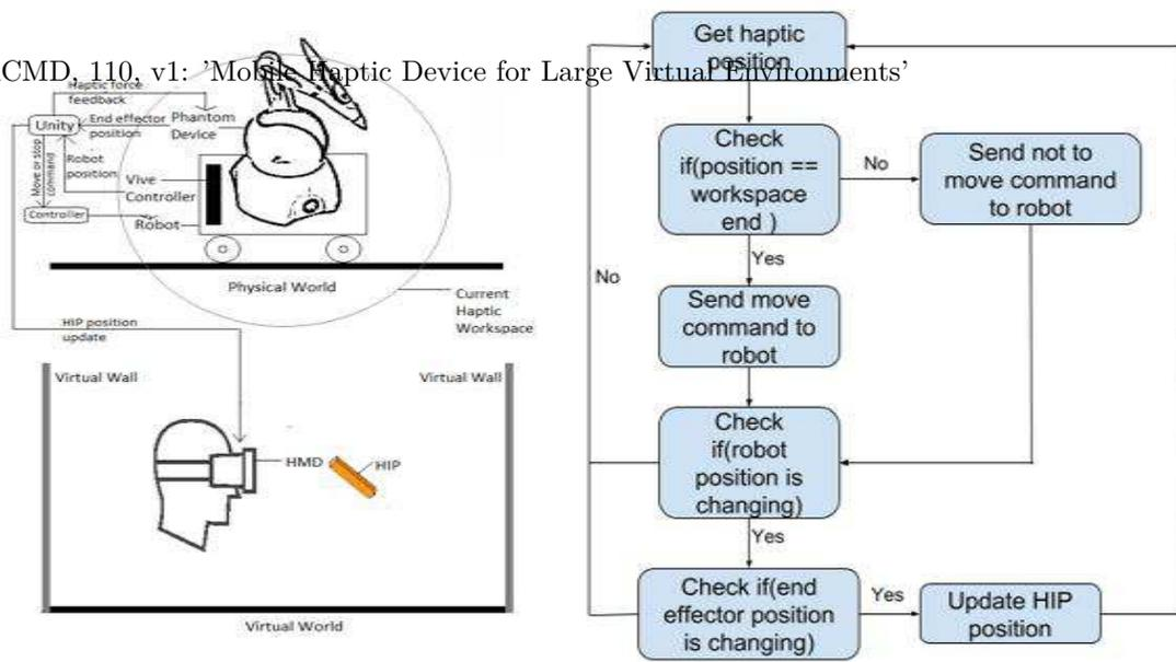
Figure 1: Device setup with the mobile robot (left) and HIP stands for Haptic Interaction Point; Position based workspace drift algorithm (right)
