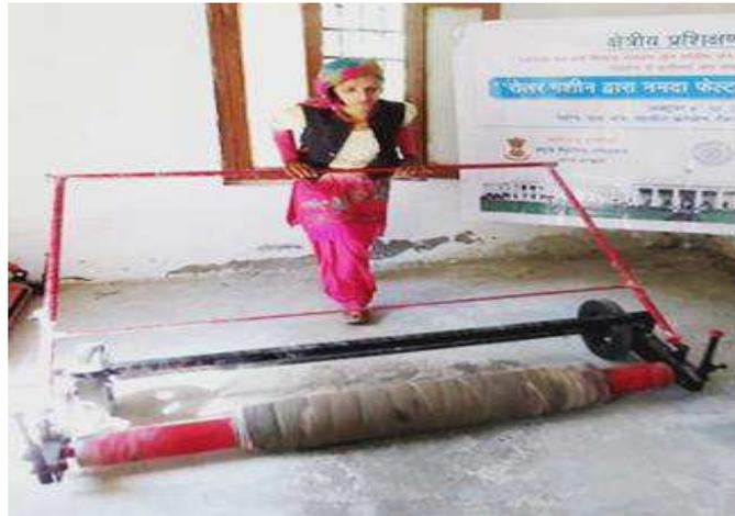
Figure 1 : Rolling felt using mechanized roller
