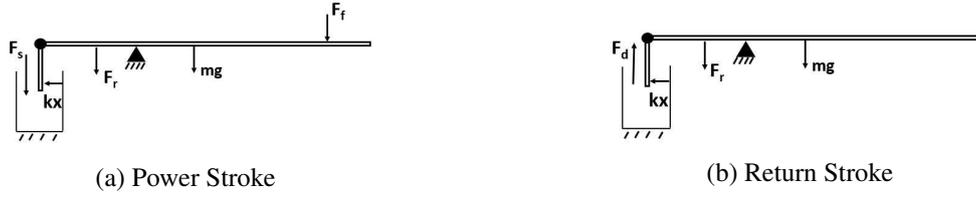
Figure 3: Forces acting on the lever during both the strokes
