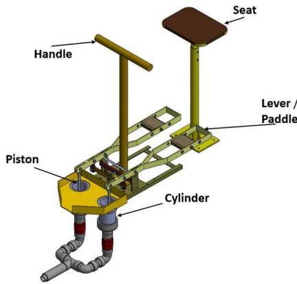
Figure 1: RuTAG Treadle Pump
