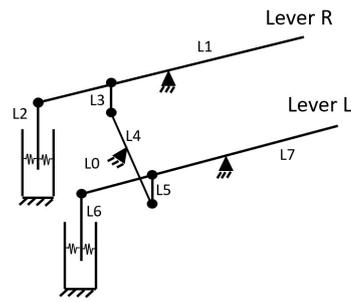
Figure 2: Line Diagram of Lever - Piston Assembly
